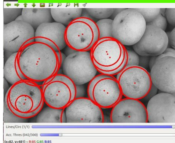
Figure 7-6. (clockwise, from top left) original image, Canny edges with a tight threshold and attempts to fit circles to the image at different Hough accumulator thresholds
